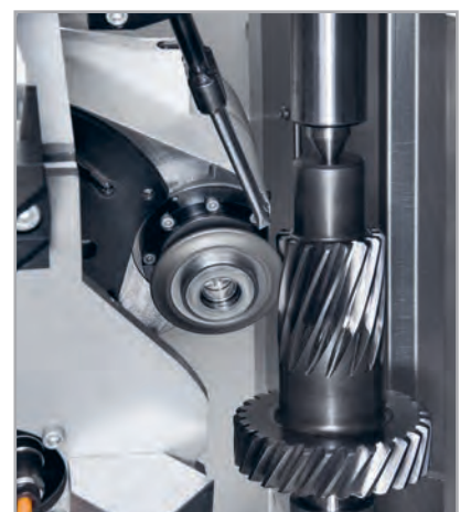
Profile grinding with profile grinding head
