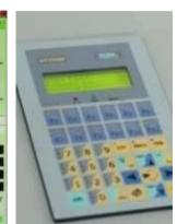
INDUCAM control and data storage of heattreatment parameters
