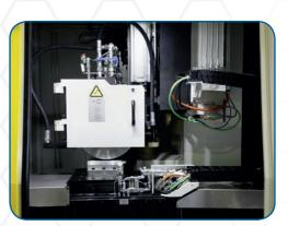
Surface grinder for high cutting speeds and high workpiece speeds with pendulum grinding function.
